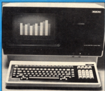
HARD MEMORY — The Memory 8000 series of micros features the normal Z80, 64K small business personal micro environment with an added attraction to make them stand out in the crowd. The operating system is a CP/M-compatible multi-user, multi-tasker called Brides. Dealer prices for the twin 400K floppy version are £1,500 and the Winchester model, with 800K on a floppy, starts at £3,400 — volume discounts apply but note that these are dealer prices.
